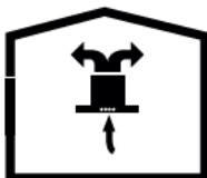
Fig. 5: Air Circulation with Carbon Filter
